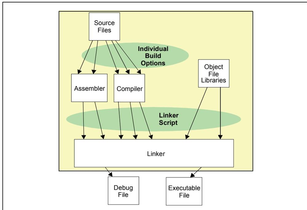
The source files are text files that are written conforming to the rules of the assembler or compiler. The assembler and compiler convert them into intermediate modules of machine code and placeholders for references to functions and data storage. The linker resolves these placeholders and combines all the modules into a file of executable machine code. The linker also produces a debug file which allows MPLAB X IDE to relate the executing machine codes back to the source files.
