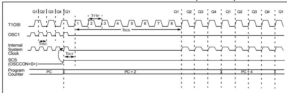
**FIGURE 1-6: PIC® MCU DATA SHEET – INSTRUCTIONS (EXCERPT)**
