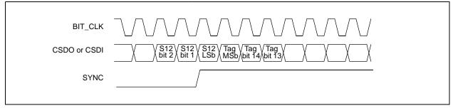
FIGURE 18-4: I<sup>2</sup>S INTERFACE FRAME SYNC TIMING
