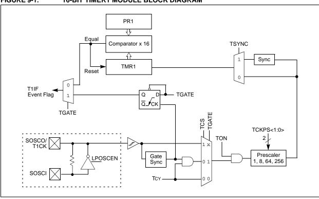
FIGURE 9-1: 16-BIT TIMER1 MODULE BLOCK DIAGRAM
