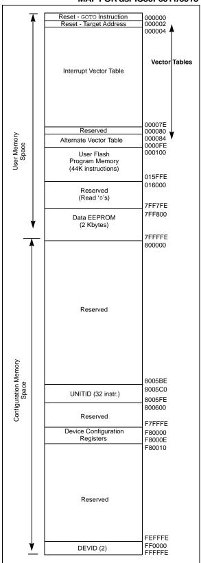
FIGURE 3-2: PROGRAM SPACE MEMORY MAP FOR dsPIC30F6012/6014
