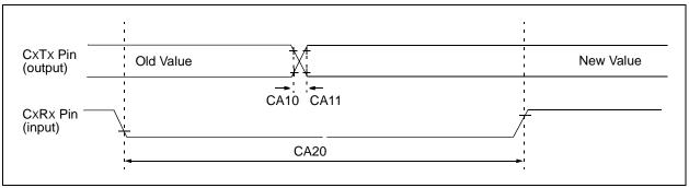
TABLE 23-37: CAN MODULE I/O TIMING REQUIREMENTS
