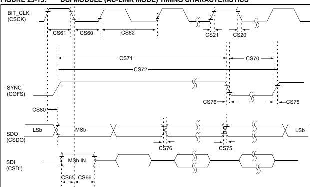
FIGURE 23-13: DCI MODULE (AC-LINK MODE) TIMING CHARACTERISTICS
