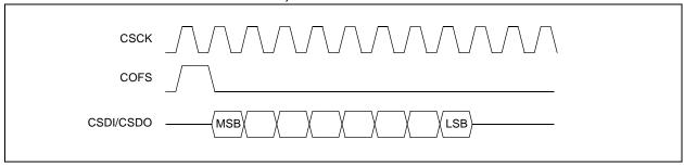
FIGURE 18-3: FRAME SYNC TIMING, AC-LINK START OF FRAME
