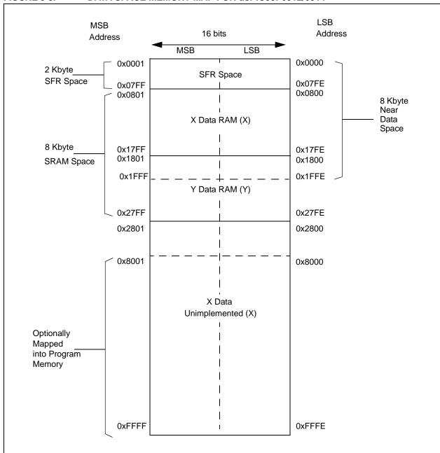
FIGURE 3-8: DATA SPACE MEMORY MAP FOR dsPIC30F6012/6014
