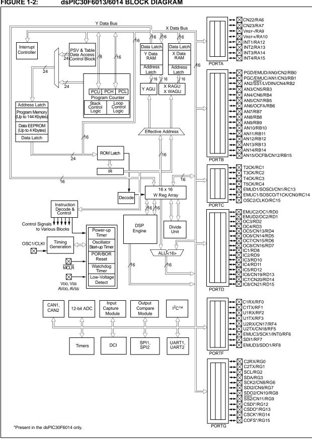
FIGURE 1-2: dsPIC30F6013/6014 BLOCK DIAGRAM
