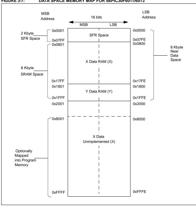
FIGURE 3-7: DATA SPACE MEMORY MAP FOR dsPIC30F6011/6013
