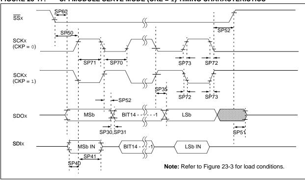
FIGURE 23-17: SPI MODULE SLAVE MODE (CKE = 1) TIMING CHARACTERISTICS
