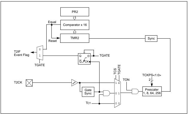
FIGURE 10-3: 16-BIT TIMER3 BLOCK DIAGRAM
