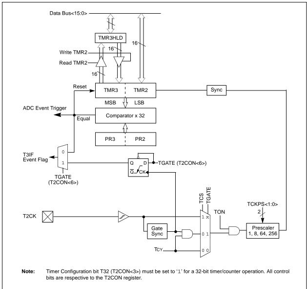
FIGURE 10-2: 16-BIT TIMER2 BLOCK DIAGRAM
