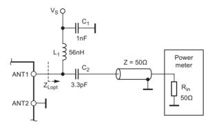
Note: For 345MHz C<sub>2</sub> has to be changed to 2.7pF
