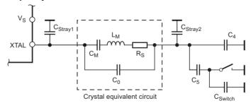
Using  $C_4$  = 8.2pF ±5%,  $C_5$  = 10pF ±5%, a switch port with  $C_{Switch}$  = 3pF ±10%, stray capacitances on each side of the crystal of  $C_{Stray1}$  =  $C_{Stray2}$  = 1pF ±10%, a parallel capacitance of the crystal of  $C_0$  = 3.2pF ±10% and a crystal with  $C_M$  = 13fF ±10%, an FSK deviation of ±21.5kHz typical with worst case tolerances of ±16.25kHz to ±28.01kHz results.
