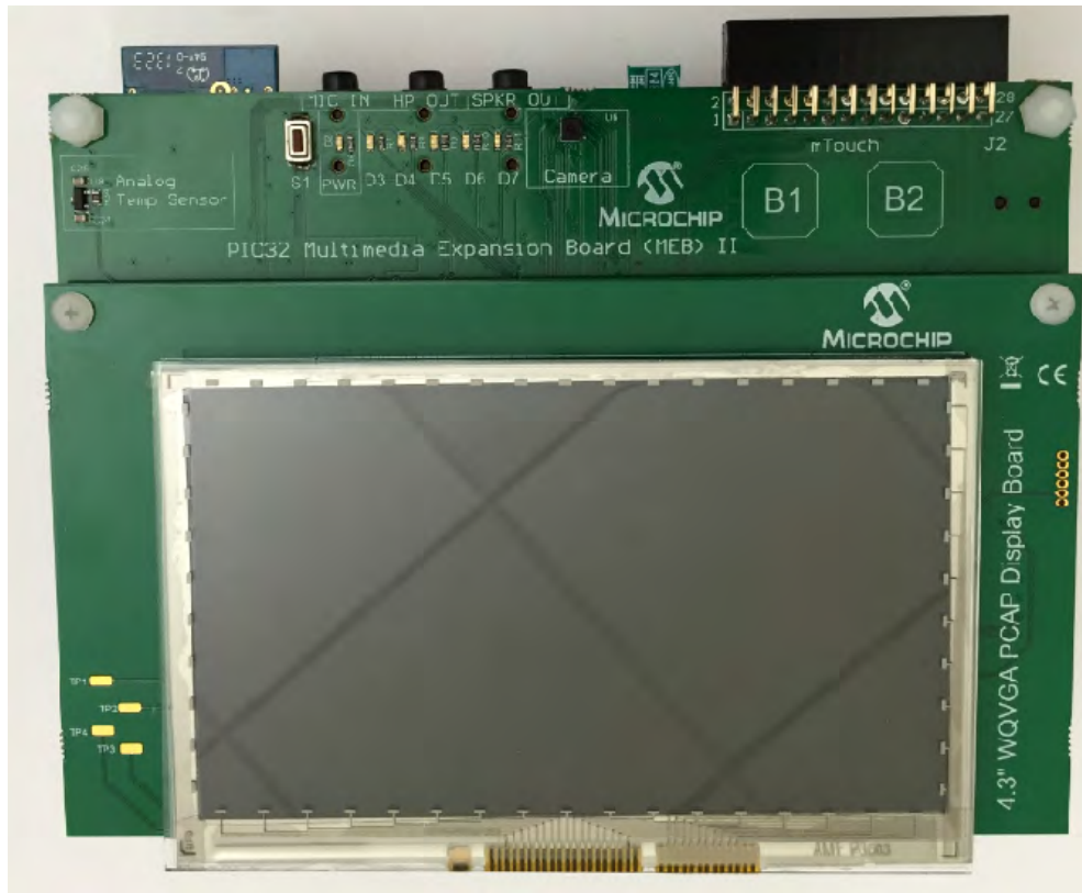
MRF24WG0MA Wi-Fi module, 4.3" WQVGA PCAP Display Board, and Multimedia Expansion Board II (MEB II) Configure the hardware, as shown in the following figures:
