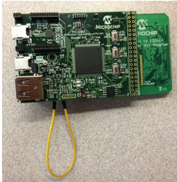
PIC32MZ EF Starter Kit and Adapter Board connected to the Graphics Controller PICtail Plus Epson S1D13517 Daughter Board
