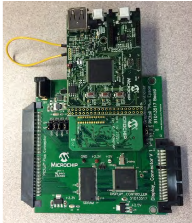
PIC32MZ EF Starter Kit and Adapter Board connected to the Graphics Controller PICtail Plus Epson S1D13517 Daughter Board
