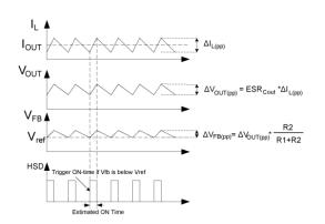
Figure 2. MIC261201 Control Loop Timing
