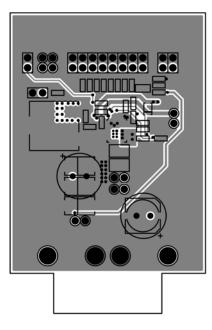
Figure 11. MIC261201 Evaluation Board Mid-Layer 2
