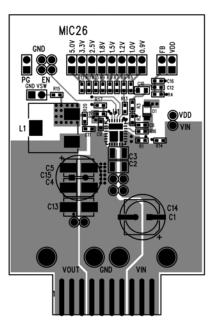
Figure 9. MIC261201 Evaluation Board Top Layer
