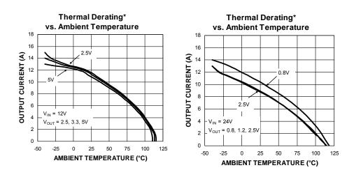
**Die Temperature\***: The temperature measurement was taken at the hottest point on the MIC261201 case mounted on a 5 square inch 4 layer, 0.62", FR-4 PCB with 2oz finish copper weight per layer, see Thermal Measurement section. Actual results will depend upon the size of the PCB, ambient temperature and proximity to other heat emitting components.
