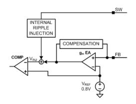
Figure 7. Internal Ripple Injection
