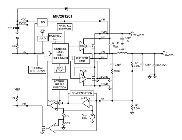
Figure 1. MIC261201 Block Diagram
