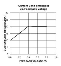
Figure 4. MIC261201 Current-Limit Foldback Characteristic
