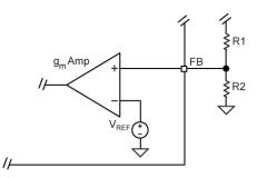
Figure 6. Voltage-Divider Configuration
