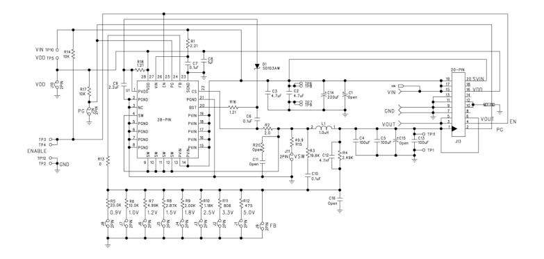
Figure 8. Schematic of MIC261201 Evaluation Board
