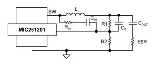
Figure 5c. Invisible Ripple at FB
