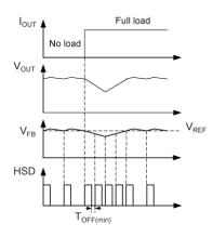
Figure 3. MIC261201 Load Transient Response
