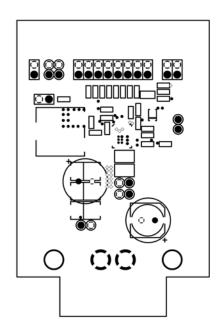
Figure 10. MIC261201 Evaluation Board Mid-Layer 1 (Ground Plane)
