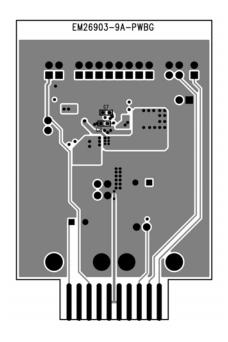
Figure 12. MIC261201 Evaluation Board Bottom Layer
