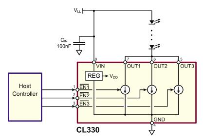
By paralleling outputs, higher LED currents can be achieved. In addition, linear dimming in 3 discrete steps may be obtained by enabling 1, 2, or 3 outputs.
