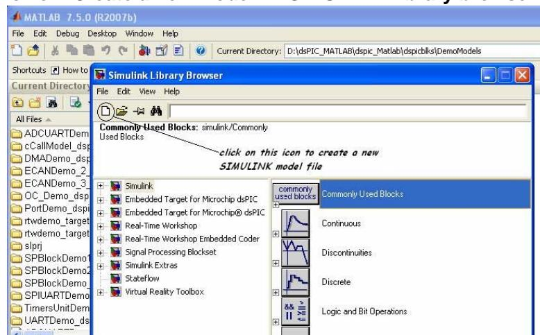
1. Click on 'Create a new Model' in SIMULINK Library browser. This would open up an empty model file. You can populate this model file with different blocks from SIMULINK library and create an application model.
