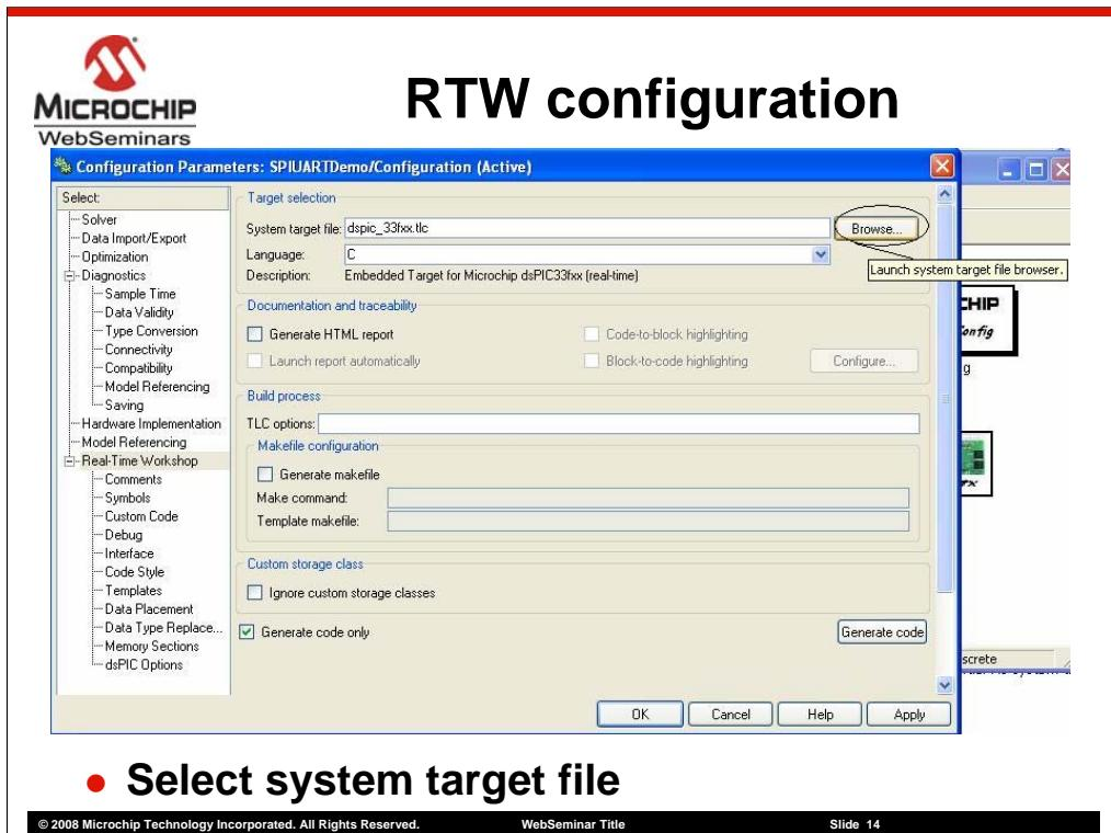
Here we have view of ‘Real Time Workshop’ pane of RTW configuration dialog. You have to choose ‘**dspic\_33fxx.tlc**’ as system target file. You can choose this file by clicking ‘Browse’ button which is circled in the picture shown. This will pop up a list of system target files that are registered in your MATLAB installation.
