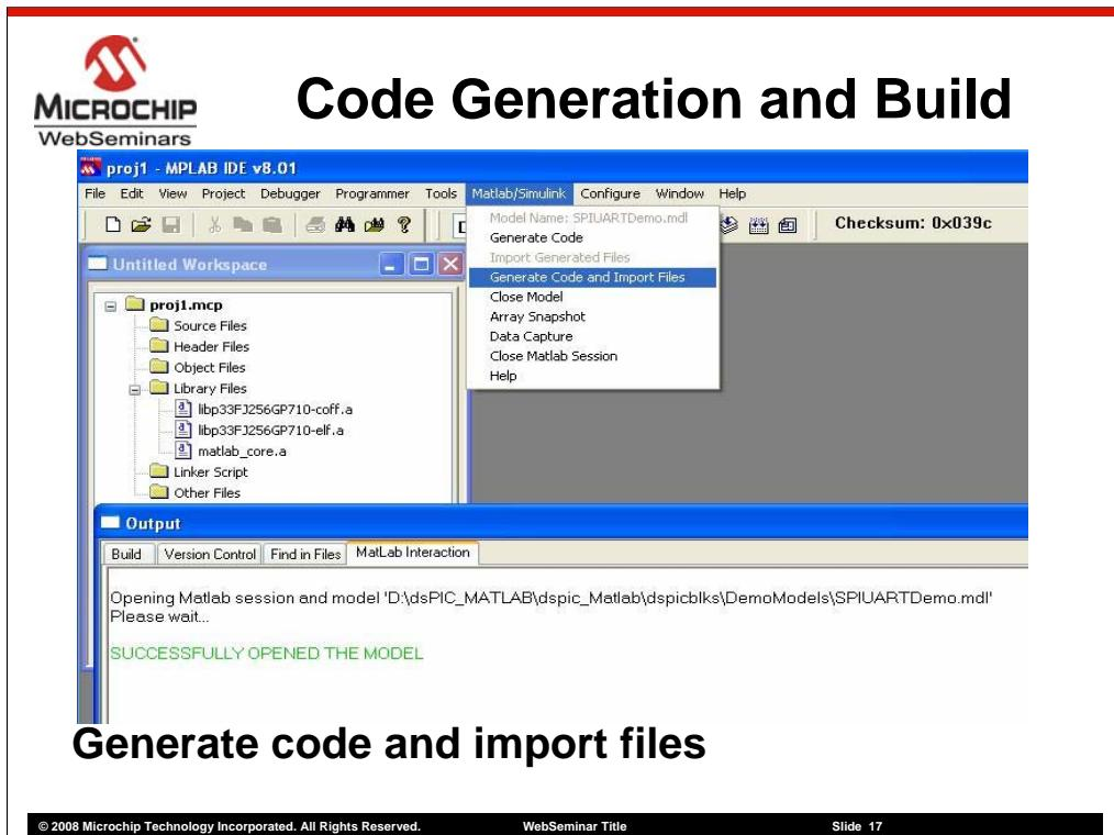
Picture here shows how to generate and import files from a SIMULINK model once you have configured RTW settings and saved the model.
