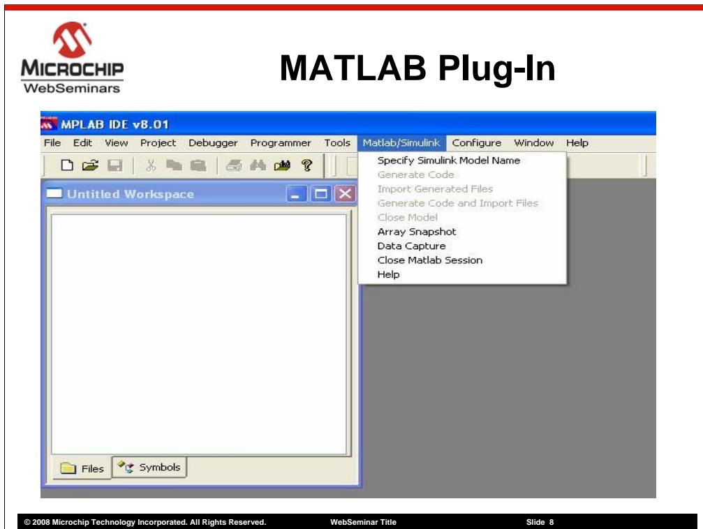
The screen shot shows the MPLAB® IDE with MATLAB/SIMULINK menu. It appears when user clicks on MATLAB/SIMULINK in ‘Tools’ drop down menu of MPLAB® IDE. When you click on ‘Specify Simulink Model name’, it will prompt the user to choose a SIMULINK model to open.
