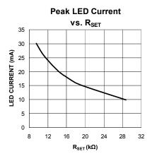
Figure 2. Peak LED current vs. R<sub>SET</sub>
