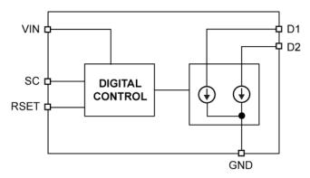
Figure 1. MIC2860-2D Functional Block Diagram
