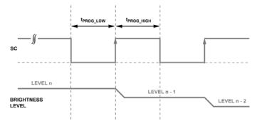
Figure 5. Brightness Programming Pulses
