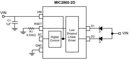
LCD Display Backlight with 2 WLEDs
