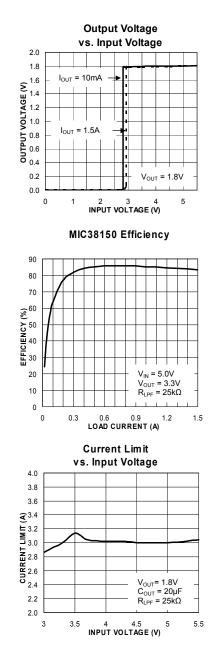
**Typical Characteristics**  $V_{IN}$  = 3.3V,  $V_{OUT}$  = 1.8V,  $C_{OUT}$  = 10µF,  $R_{LPF}$  = 25k $\Omega$ ,  $I_{OUT}$  = 100mA, unless noted
