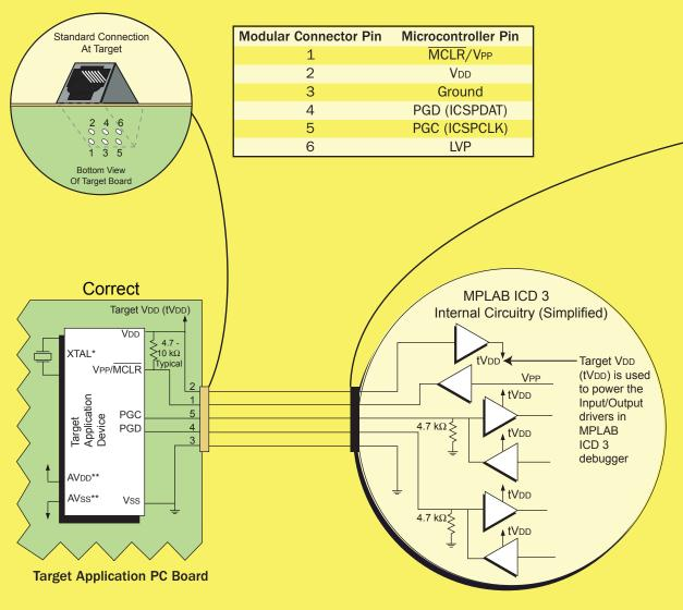
\*Target device must be running with an oscillator for the debugger to function as a debugger.
