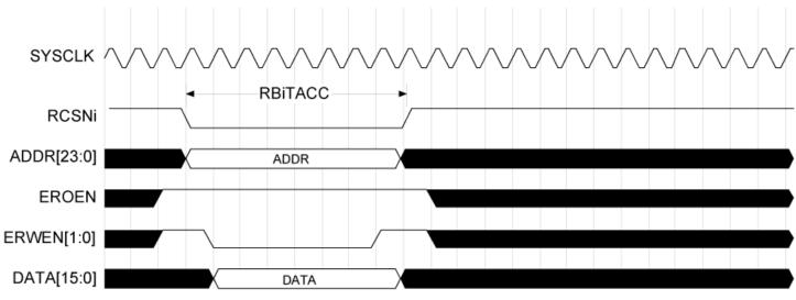
Figure 18. Static Memory Write Cycle
