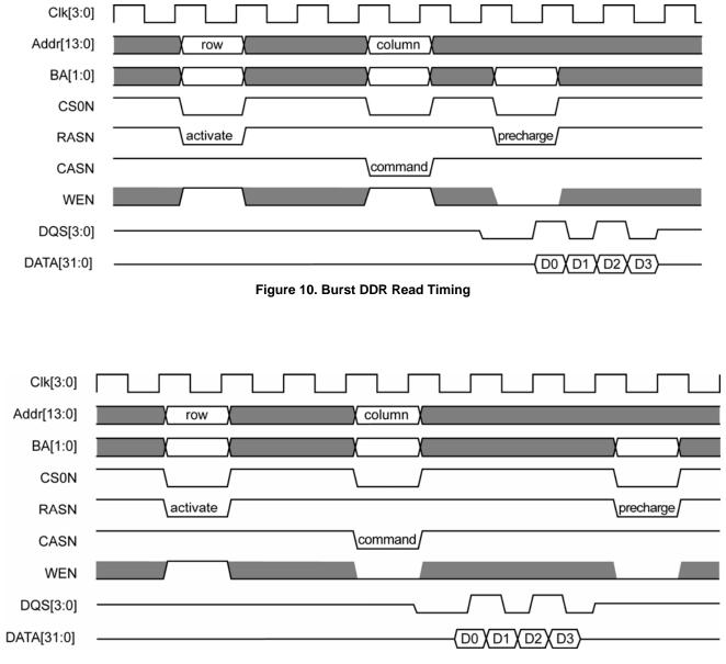
Figure 11. Burst DDR Write Timing
