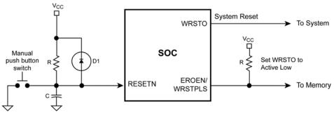
Figure 14. Reset Circuit
