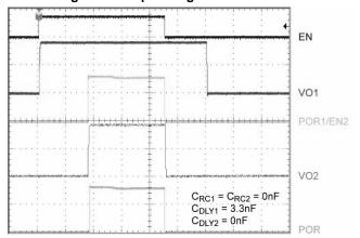
Figure 5. Window Sequencing Example
