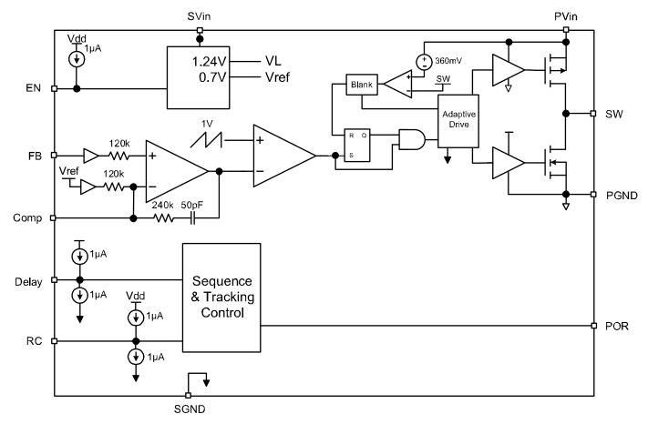
Figure 1. MIC22600 Block Diagram
