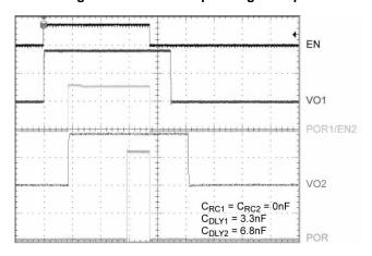
Figure 6. Delayed Sequencing Example
