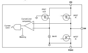
Figure 13. Current-Limit Detail
