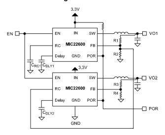
Figure 9. Ratio Metric Tracking Circuit
