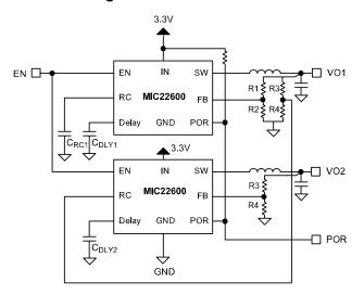
Figure 7. Normal Tracking Circuit
