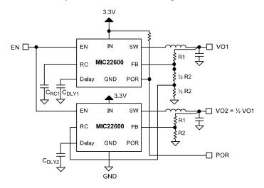
Figure 11. DDR Memory Tracking Circuit
