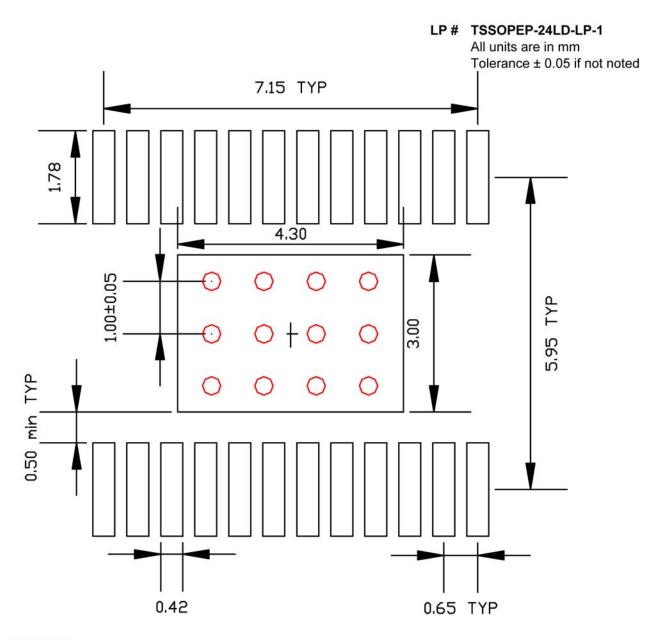
Red circle indicates Thermal Via. Size should be .300mm - .350mm in diameter, and it should be connected to GND plane for maximum thermal performance.
