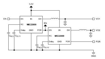
Figure 4. Sequencing MIC22600 Circuit
