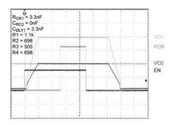
Figure 12. DDR Memory Tracking Example
