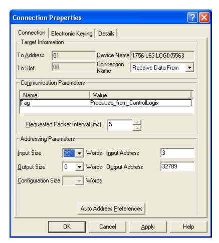
11. Double click the *Value* field and enter the produced tag name created in RSLogix5000. Enter the *Input Size*, which should be the size of the produced tag defined earlier in RSLogix5000. Note: this size is in words, whereas the size of the user defined data type shown in RSLogix5000 is in bytes. Set the *Requested Packet Interval*, in ms; the minimum possible value is the NUT. Click *Apply*, then *OK*.
