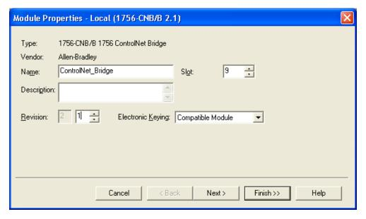
9. Right click on the bridge module just added and select *New Module*. Highlight the entry for a ControlNet PLC5 – *1785-PLC5C ControlNet PLC5* – and click *OK*.
