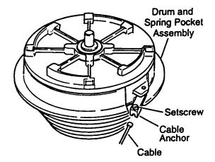
NOTE: Cable must be fully wound onto drum before attaching rear case.
