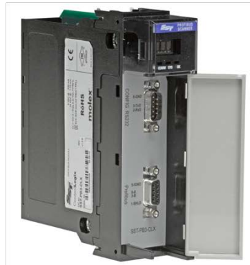
SST-PB3S-CLX-RLL-CC Conformal Coated version
