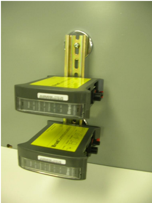
Figure 8: Remote Scanners, Mounted Horizontally
