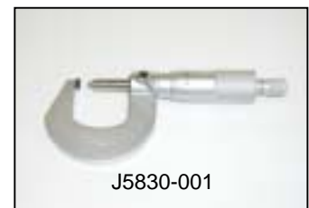
Measurement of crimp height of conductor wire
