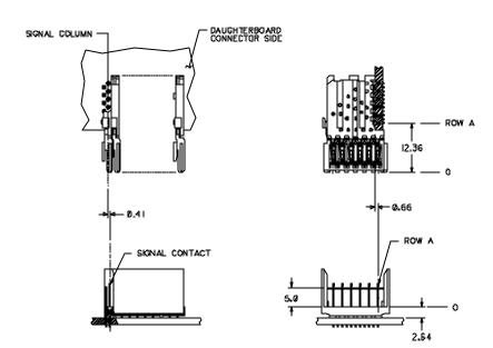
2.00 by 2.25mm (.079 by .089") Pitch VHDM® Backplane Connector System
