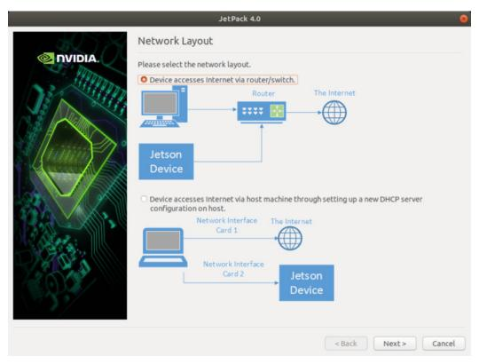
11. If you selected the **Device access Internet via router/switch** layout, you will be asked to select which interface to use for Internet access.
