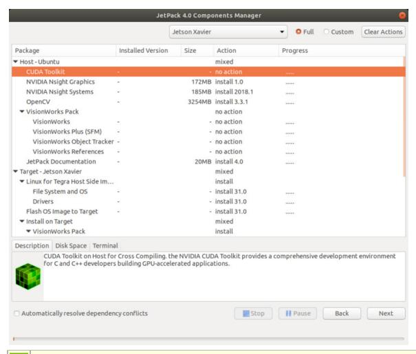
NOTE: To run a standalone Ubuntu install, deselect Jetson target specific entries.
