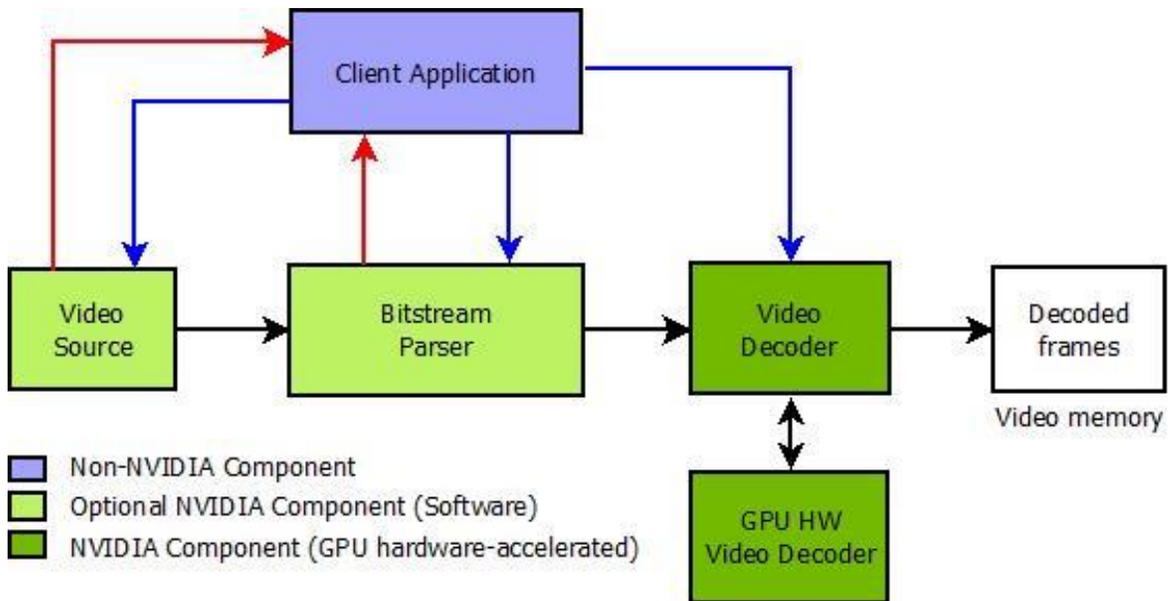
Figure 1. Video decoder pipeline using NVDECODE API
