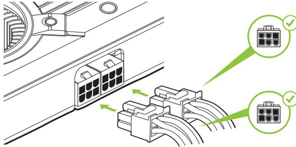
If your power supply needs an additional power connector, you can use the included 4-to-6 pin adapter.
