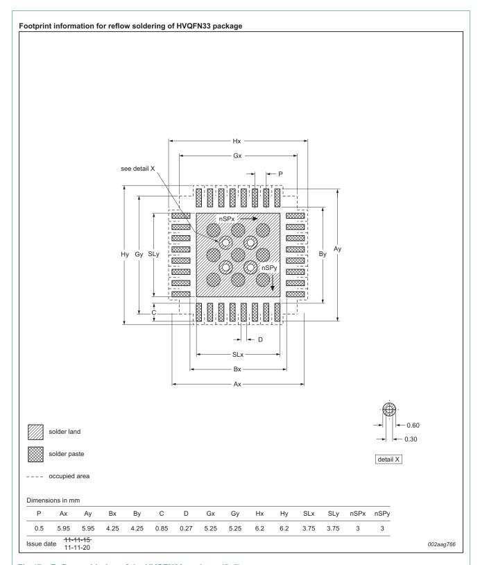
Fig 47. Reflow soldering of the HVQFN33 package (5x5)
