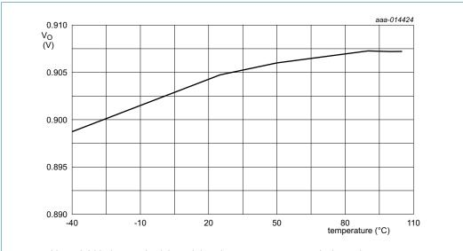
$V_{DD}$  = 3.3 V; characterized through bench measurements on typical samples.
