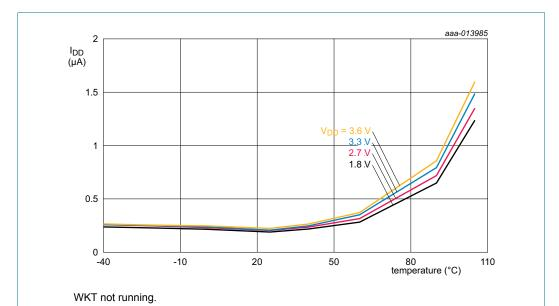
Fig 18. Deep power-down mode: Typical supply current I<sub>DD</sub> versus temperature for different supply voltages V<sub>DD</sub>
