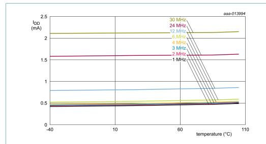
Conditions:  $V_{DD} = 3.3 \text{ V}$ ; sleep mode entered from flash; all peripherals disabled in the SYSAHBCLKCTRL register (SYSAHBCLKCTRL =0x1F); all peripheral clocks disabled; internal pull-up resistors disabled; BOD disabled; low-current mode.
