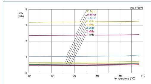
Conditions:  $V_{DD}$  = 3.3 V; active mode entered executing code while(1){} from flash; all peripherals disabled in the SYSAHBCLKCTRL register (SYSAHBCLKCTRL =0x1F); all peripheral clocks disabled; internal pull-up resistors disabled; BOD disabled; low-current mode.
