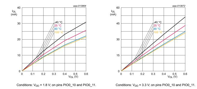
Fig 26. I<sup>2</sup>C-bus pins (high current sink): Typical LOW-level output current I<sub>OL</sub> versus LOW-level output voltage VoL
