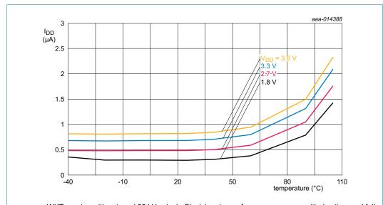
WKT running with external 32 kHz clock. Clock input waveform: square wave with rise time and fall time of  $5\,\mathrm{ns}$ .
