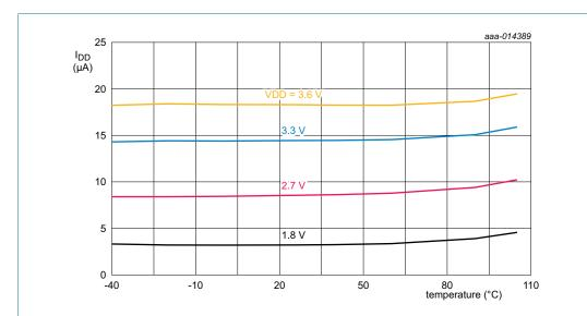
WKT running with external 1 MHz clock. Clock input waveform: square wave with rise time and fall time of  $5\,\mathrm{ns}$ .
