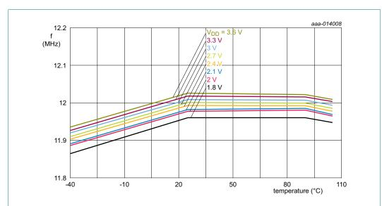
Conditions: Frequency values are typical values. 12 MHz  $\pm$  1.5 % accuracy is guaranteed for 2.7 V  $\leq$  V<sub>DD</sub>  $\leq$  3.6 V. Variations between parts may cause the IRC to fall outside the 12 MHz  $\pm$  1.5 % accuracy specification for voltages below 2.7 V.
