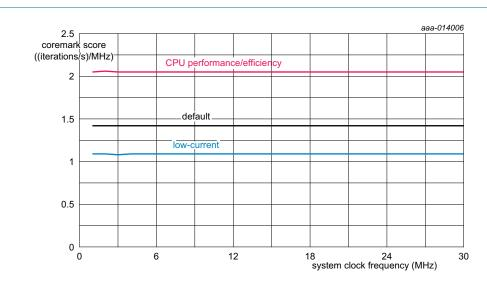
Conditions:  $V_{DD}$  = 3.3 V;  $T_{amb}$  = 25 °C; active mode; all peripherals except one UART and the SCT disabled in the SYSAHBCLKCTRL register; BOD disabled; internal pull-up resistors enabled. Measured with Keil uVision 5.10.
