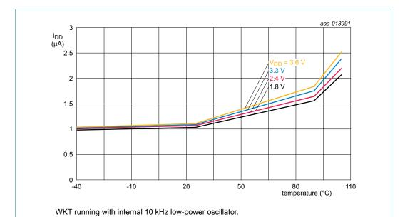
Fig 19. Deep power-down mode: Typical supply current I<sub>DD</sub> versus temperature for different supply voltages V<sub>DD</sub> (internal clock)
