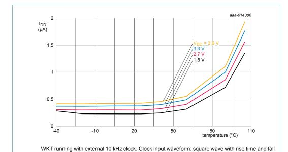
Fig 20. Deep power-down mode: Typical supply current I<sub>DD</sub> versus temperature for different supply voltages V<sub>DD</sub> (external 10 kHz input clock)
