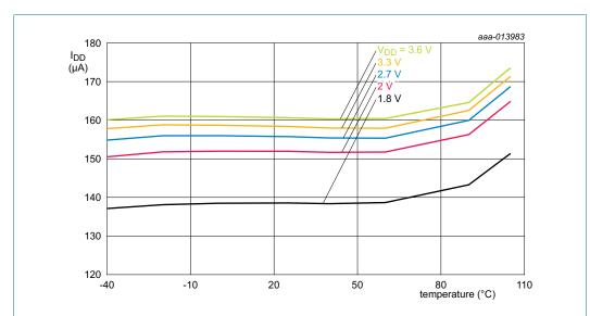
Conditions: BOD disabled; all oscillators and analog blocks disabled in the PDSLEEPCFG register (PDSLEEPCFG = 0x0000 18FF).
