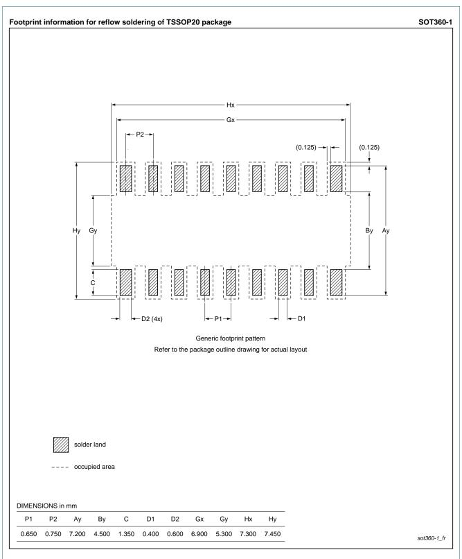
Fig 46. Reflow soldering of the TSSOP20 package
