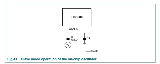
In slave mode the input clock signal should be coupled with a capacitor of 100 pF (Figure 41), with an amplitude between 200 mV (RMS) and 1000 mV (RMS). This corresponds to a square wave signal with a signal swing of between 280 mV and 1.4 V. The XTALOUT pin in this configuration can be left unconnected.
