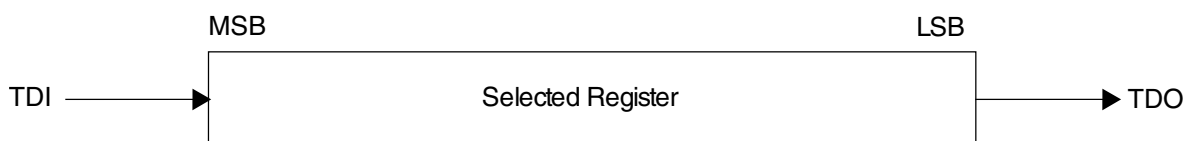
Figure 48-3. Shifting data through a register
