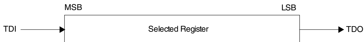
Figure 51-3. Shifting data through a register
