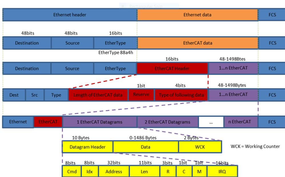
Figure 58. EtherCAT frame structure
