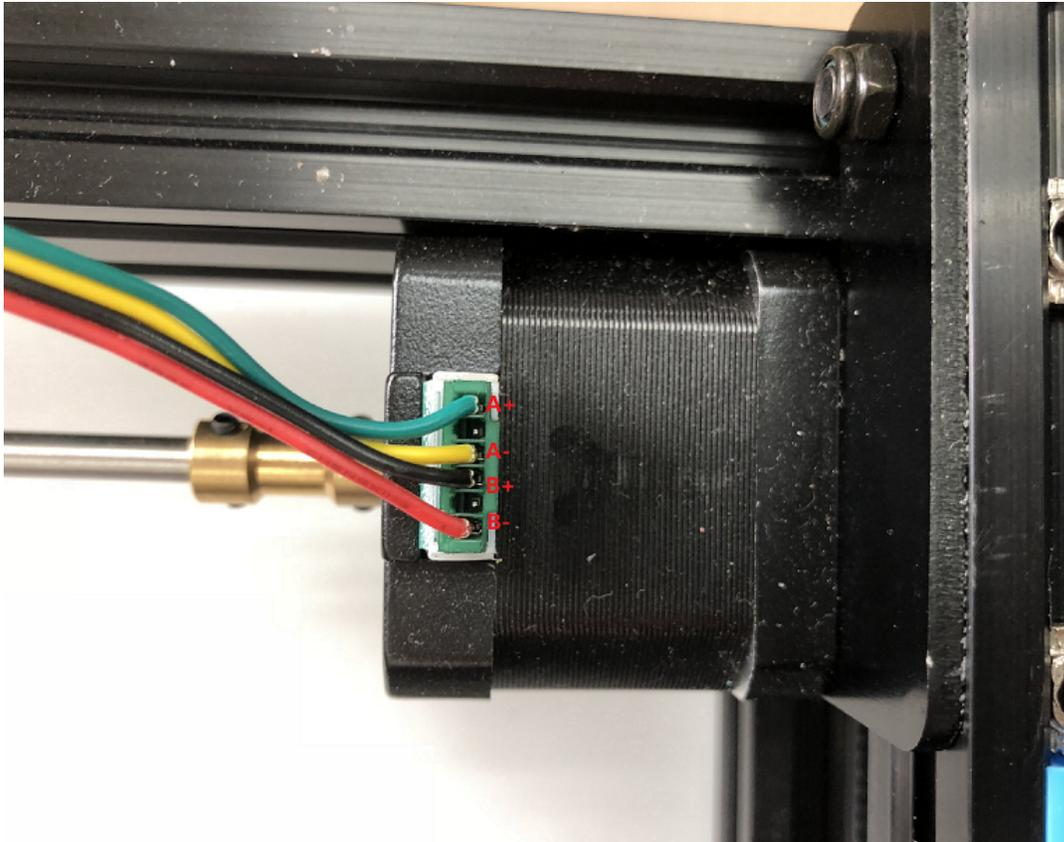
**Figure 62. Stepper motor**
