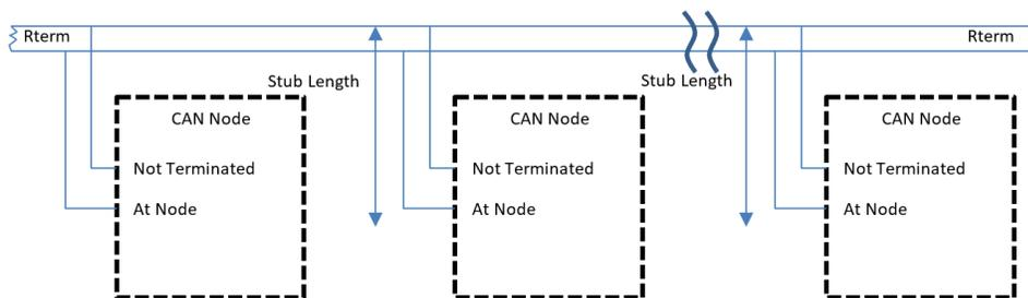
Figure 66. High speed CAN network
