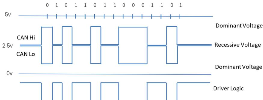
Figure 64. High speed CAN signaling
