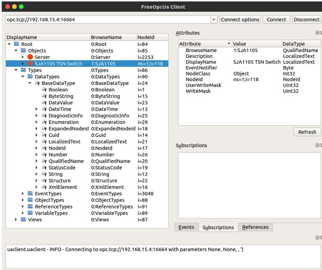
Shown on the left-hand side of the figure is the *Address Space* (collection of information that the server makes available to clients) of the OPC server found at `opc.tcp://192.168.15.4:16664`.
