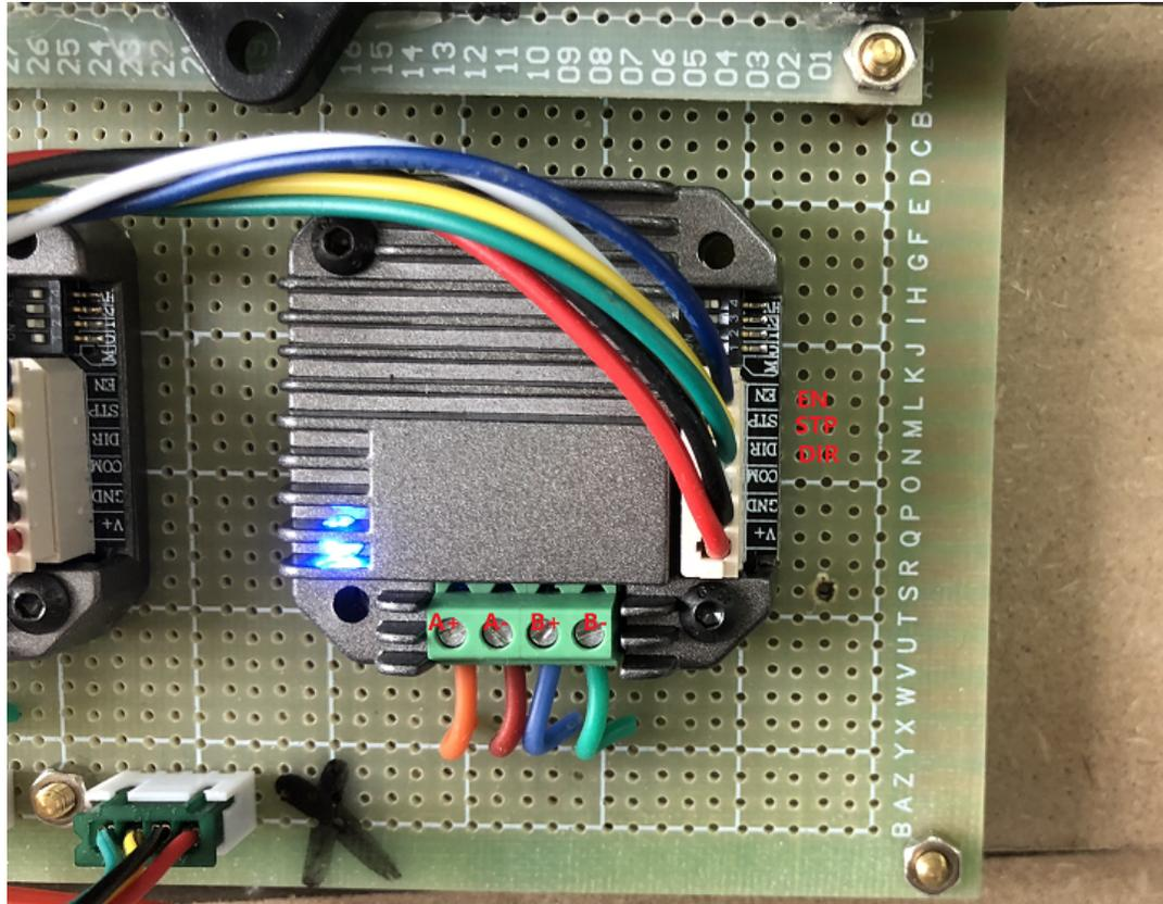
**Figure 61. Stepper motor driver**
