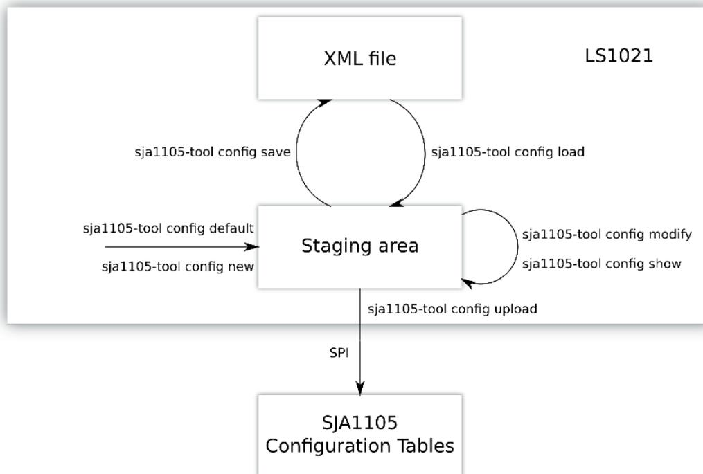
The physical SPI registers of the SJA1105 switch are write-only. Therefore, a copy of these registers is kept in the staging area, which is effectively a file in the LS1021A OpenIL filesystem. The staging area keeps a binary image of the configuration to be uploaded over SPI using `sja1105-tool config upload`, and can also be read back by the user with `sja1105-tool config show`.
