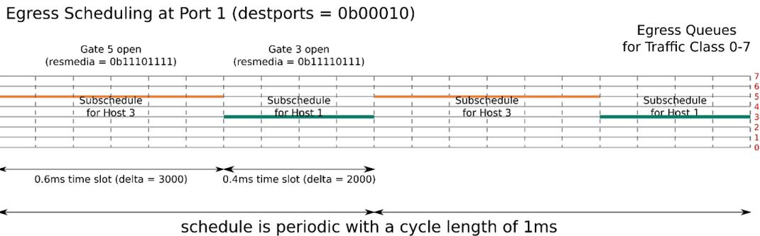
**Figure 45. Time gating for Host 1 and Host 3, viewed on the time axis**
