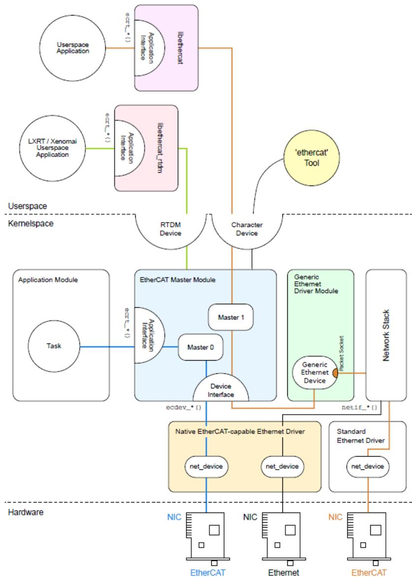
Figure 57. IGH EtherCAT master architecture
