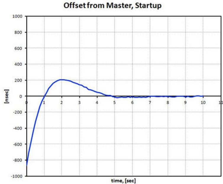
Figure 6. Offset from master in start up state
