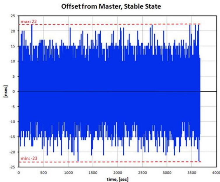
Figure 7. Offset from master in stable state
