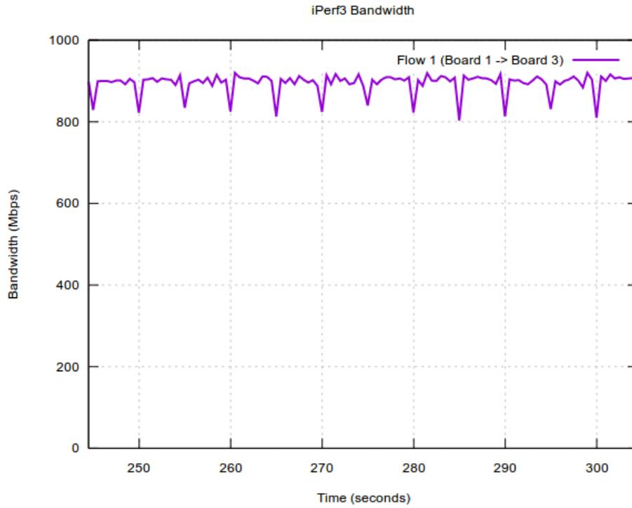
**Figure 37. Prioritizing configuration: Flow 1 run by its own**
