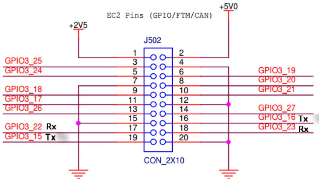
Figure 68. Hardware diagram for the FlexCan demo
