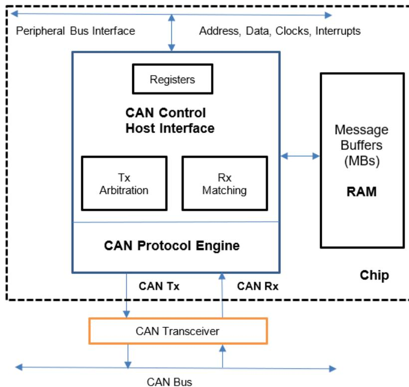
Figure 63. FlexCAN block diagram
