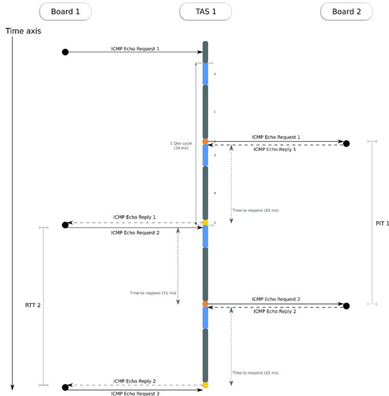
On the time axis, on the left hand side are Round-Trip Times (RTT) reported by Node A (sender), while on the right-hand side are Packet Interarrival Times (PIT) reported by Node B (receiver).
