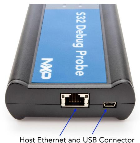
Figure 11. S32 Debug Probe - Ethernet and USB connector
