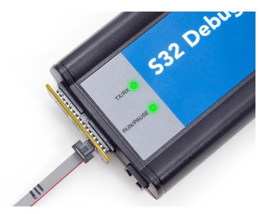
Figure 10. S32 Debug Probe - LED indicators
