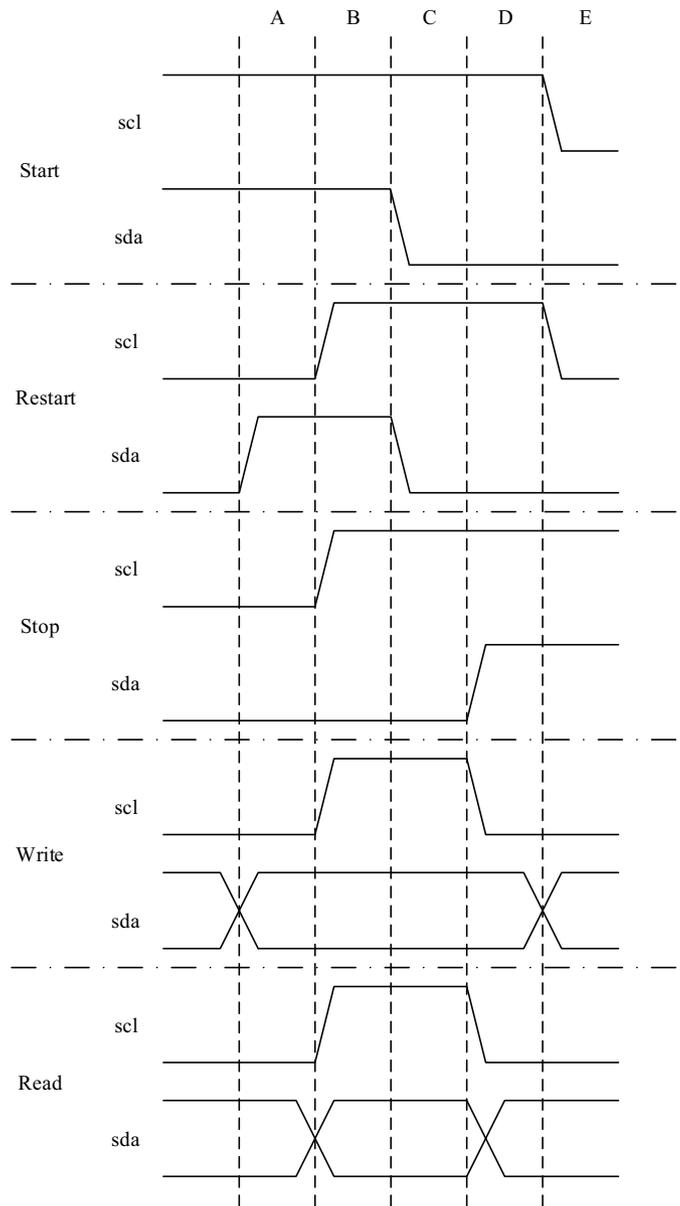
Fig 7. Bit waveform
