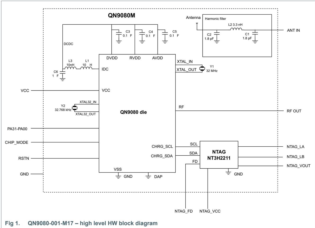
Fig 1. QN9080-001-M17 – high level HW block diagram
