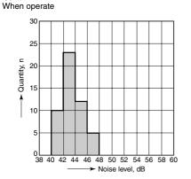
6.-(2)-2 Operation noise distribution (horizontal type) When release
