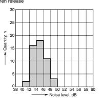
Horizontal type Measuring conditions Sample: AEVS960122, 50pcs Equipment setting: "A" weighted, Fast, Max. hold Coil voltage: 12 V DC Coil connection device: 18 V zener diode Background noise: approx. 20dB
