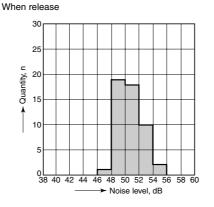
Vertical type Measuring conditions Sample: AEVS16012, 50pcs Equipment setting: "A" weighted, Fast, Max. hold Coil voltage: 12 V DC Coil connection device: 18 V zener diode Background noise: approx. 20dB
