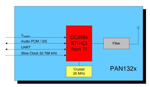
Note: The Slow Clock 32.768 kHz is mandatory, otherwise the module does not start up, refer to Chapter 6.4 for additional information.
