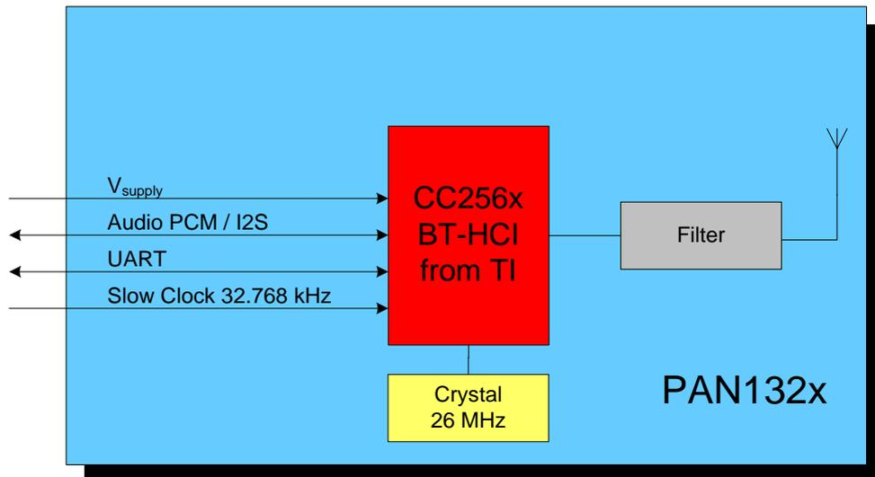
Note: The Slow Clock 32.768 kHz is mandatory, otherwise the module does not start up, refer to Chapter 6.4 for additional information.
