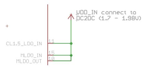
3. Mixed DC2DC- $V_{BAT}$  system (Maximum RF output power and optimum system power, but requires routing of  $V_{BAT}$ ):
