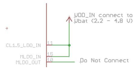
2. Full-DC2DC system (Lower RF output power, but optimum system power):
