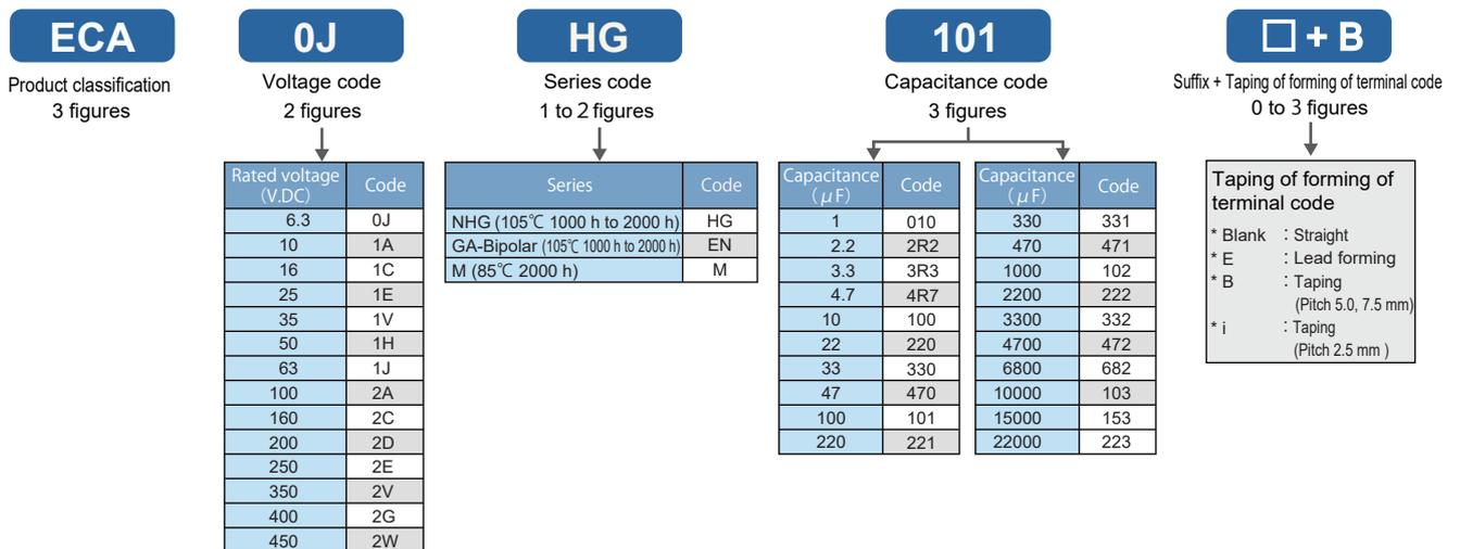
◇ Type 3 (Series : KA, KA-Bipolar, KS, KS-Bipolar, SU-Bipolar)
