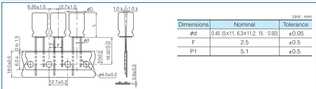
**Figure D** (Lead space: 5 mm /  $\phi D \times L$  :  $\phi 5 \times 11$ ,  $\phi 6.3 \times 11.2$ , 15)
