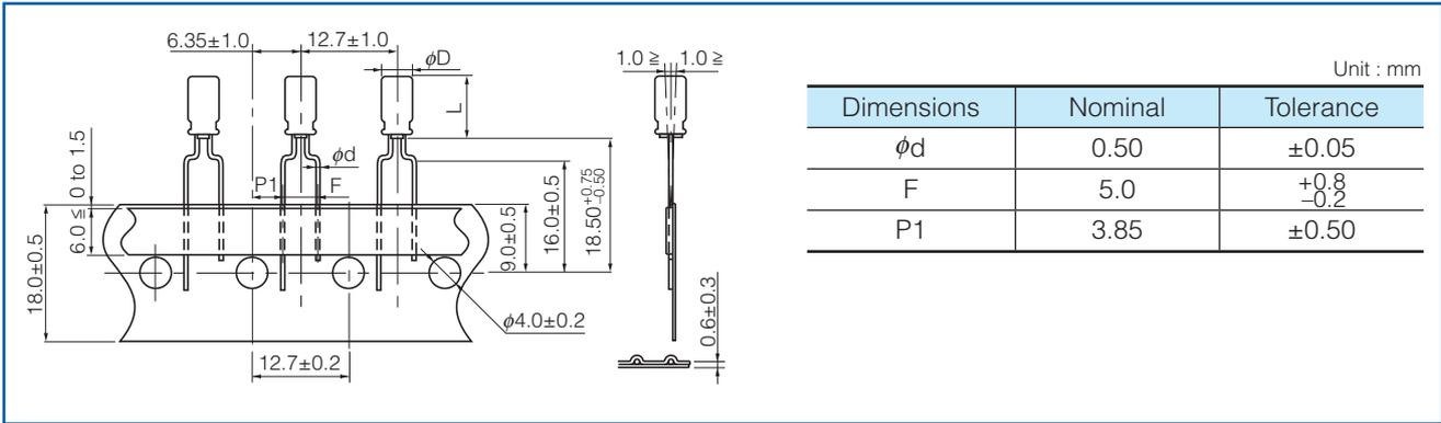
**Figure E** (Lead space: 5 mm /  $\phi D \times L$  :  $\phi 8 \times 5$ , 7, 11.5, 15, 20)
