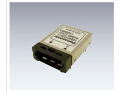
Transfer rate: 4Mbps. Compact size achived by custom IC, Builtin ATC Circuit. JIS F07 Connector adopted.
