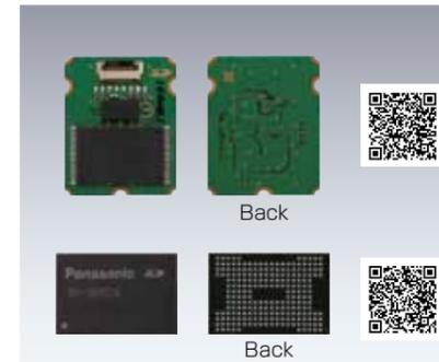
Suitable for an embedded-use. Available in 4/8/16GB. (16GB : flexible connection type only). Made in Japan.
