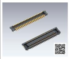
0.35 to 0.4mm terminal pitch, 1.7 to 3.6 width, and 0.6 to 1.5mm mated height. Strong resistance to advanced environments with "TOUGH CONTACT" construction.
