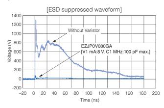
\* IEC61000-4-2 ··· International Standard of the ESD testing method (HBM) for electronic equipment ability to withstand ESD generated from a human body. It sets 4 levels of severity
