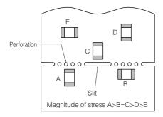
(3) The magnitude of mechanical stress applied to the Varistors when dividing the circuit board in descending order is as follows: push back < slit < V-groove < perforation. Also take into account the layout of the Varistors and the dividing/breaking method.
