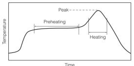
For soldering (Example: Sn-37Pb)
