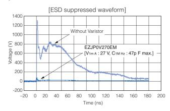
\* IEC61000-4-2 ··· International Standard of the ESD testing method (HBM) for electronic equipment ability to withstand ESD generated from a human body. It sets 4 levels of severity
