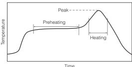
For soldering (Example : Sn-37Pb)
