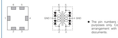
The pin numbers shown here are for reference purposes only. Confirm the actual pin number arrangement with the exchanged specification documents
