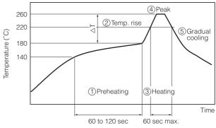
$\triangle T$ : Allowable temperature difference  $\triangle T \le 150$  °C
