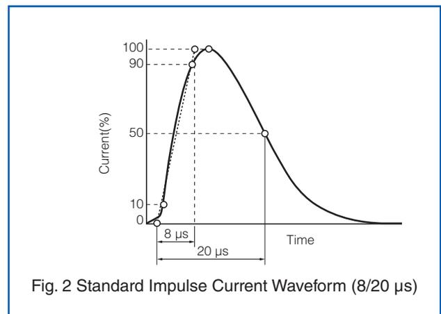
Fig. 2 Standard Impulse Current Waveform (8/20 μs)
