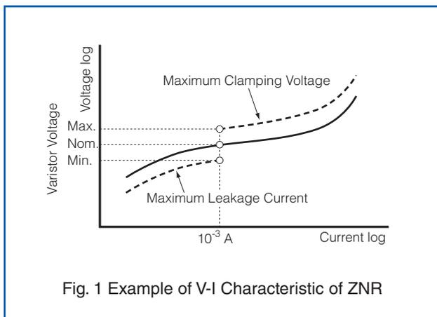
Fig. 1 Example of V-I Characteristic of ZNR
