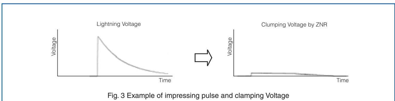
Fig. 3 Example of impressing pulse and clamping Voltage
