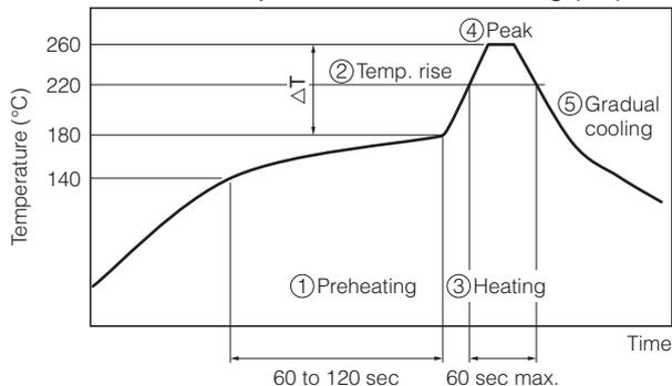
$\Delta T$  : Allowable temperature difference  $\Delta T \leq 150 \text{ }^{\circ}\text{C}$
