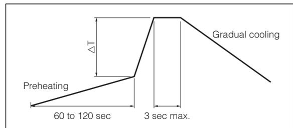
$\Delta T$  : Allowable temperature difference  $\Delta T \leq 150 \text{ }^\circ\text{C}$
