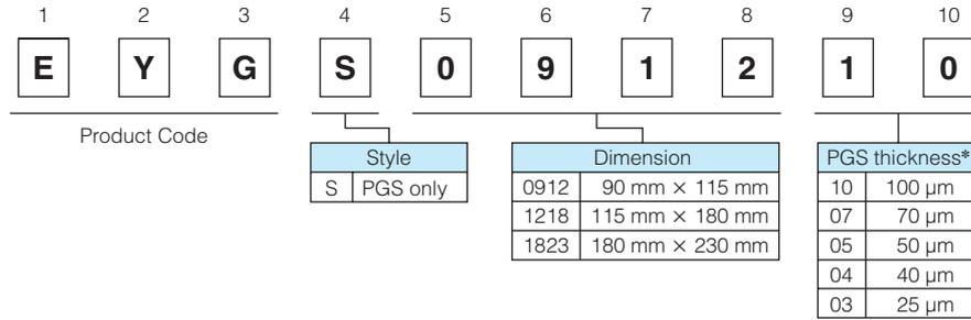
\* PGS thickness of 17 μm, 10 μm does not support as single item.
