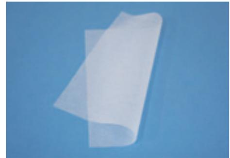
Furthermore, combining NASBIS and PGS Graphite Sheet enables controlling the direction of heat. Composite type provides greater heat insulating performance.
