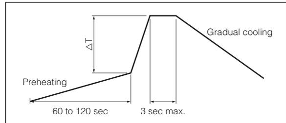
$\Delta T$  : Allowable temperature difference  $\Delta T \leq 150 \text{ }^{\circ}\text{C}$
