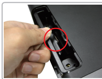
Step 2. Lift up the disk tray and pull it out gently.
