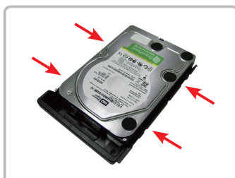
Step 3. Install a hard drive on the disk tray and lock it with four screws.
