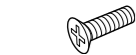
Screw used to attach the touch overlay kit (M4 x L10) 31EA Vis de fixation du kit de recouvrement tactile (M4 x L10) 31EA
