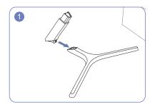
Insert the stand neck into the stand base in the direction shown in the figure. Check that the stand neck is firmly connected.
