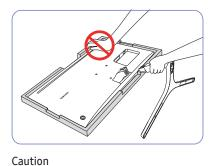
Do not press down on the monitor. There is a risk of damaging the monitor.
