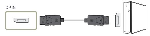
To display 3440 x 1440 @ 75 Hz, use a DP cable that supports 3440 x 1440 @ 75 Hz. Make sure that the graphics card of the DP source supports 3440 x 1440 @ 75 Hz.
