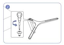
Turn the connecting screw at the bottom of the stand base to separate it.
