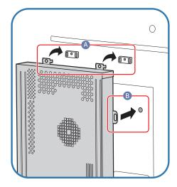
First insert the tabs of the network box into the slots marked (A) on the attachment frame. The tabs should hook onto the frame. Then, align the holes marked (B).
