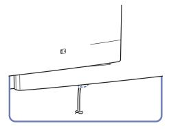
2 Insert the connected power cable through the groove.
