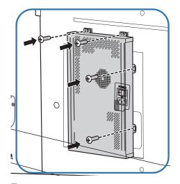
3 Attach the network box to the fixed attachment frames.
