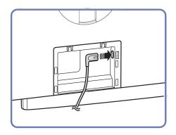
1 Connect the power cable to the power port on the back of the product.
