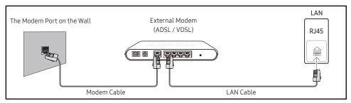
You can attach your product to your LAN by connecting the LAN port on the back of your product to an IP Sharer which is connected to an external modem. Use LAN cable for the connection. See the diagram below.
