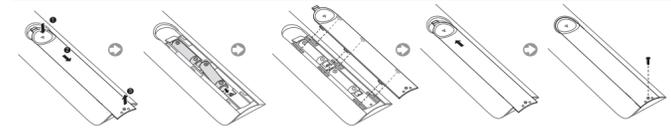
After you have installed the batteries, use a screwdriver to screw in the screw that holds the battery cover closed.
