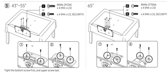
Tight the bottom screw first, and upper screw last.
