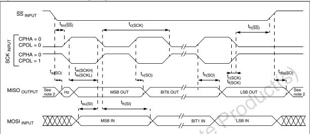
Figure 140. SPI Master Timing Diagram<sup>1)</sup>
