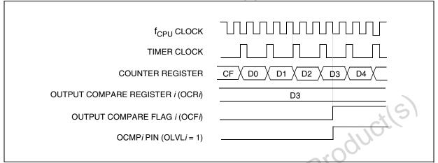
Figure 67. Output Compare Timing Diagram, f<sub>TIMER</sub> = f<sub>CPU</sub>/4
