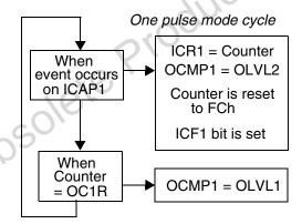
Then, on a valid event on the ICAP1 pin, the counter is initialized to FCh and OLVL2 bit is loaded on the OCMP1 pin, the ICF1 bit is set and the value FFFDh is loaded in the IC1R register.
