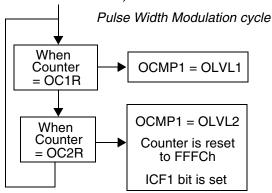
If OLVL1 = 1 and OLVL2 = 0 the length of the positive pulse is the difference between the OC2R and OC1R registers.
