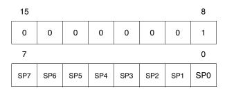
The Stack Pointer is a 16-bit register which is always pointing to the next free location in the stack. It is then decremented after data has been pushed onto the stack and incremented before data is popped from the stack (see Figure 9).
