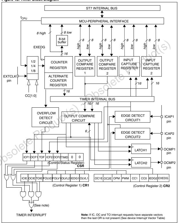
**16-bit read sequence:** (from either the Counter Register or the Alternate Counter Register).
