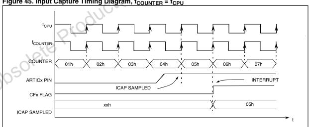
Figure 45. Input Capture Timing Diagram, f<sub>COUNTER</sub> = f<sub>CPU</sub>
