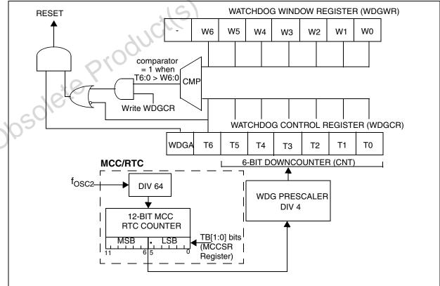
The application program must write in the WDGCR register at regular intervals during normal operation to prevent an MCU reset. This operation must occur only when the counter value is lower than the window register value. The value to be stored in the WDGCR register must be between FFh and C0h (see Figure 2):
