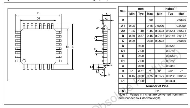
Figure 149. 32-Pin Low Profile Quad Flat Package (7x7)
