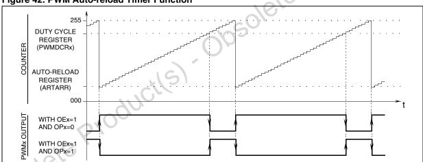
Figure 42. PWM Auto-reload Timer Function
