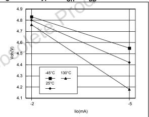
Figure 129. Typical V<sub>OL</sub> at V<sub>DD</sub> = 5V (High-sink)
