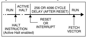
Figure 28. ACTIVE HALT Mode Flow-chart
