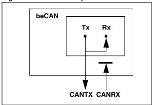
This mode is provided for self-test functions. To be independent of external events, the CAN Core ignores acknowledge errors (no dominant bit sampled in the acknowledge slot of a data / remote frame) in Loop Back Mode. In this mode, the be-CAN performs an internal feedback from its Tx output to its Rx input. The actual value of the CAN-RX input pin is disregarded by the beCAN. The transmitted messages can be monitored on the CANTX pin.
