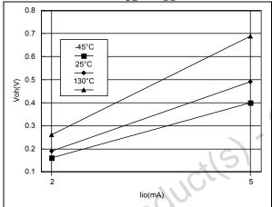
Figure 130. Typical  $V_{OH}$  at  $V_{DD} = 5V$
