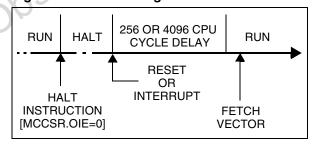
Figure 26. HALT Mode Flow-chart
