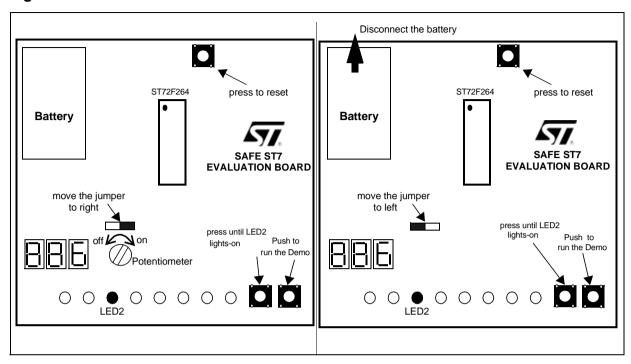
In case of power drop, and before going into reset state, the AVD interrupt will save the last displayed value in the external EEPROM (M24C08) using the I<sup>2</sup>C protocol. On power-on, the software checks if the last reset was made by the LVD, if this is the case, it downloads the previously saved value from the external EEPROM to RAM memory in order to resume counting as normal.
