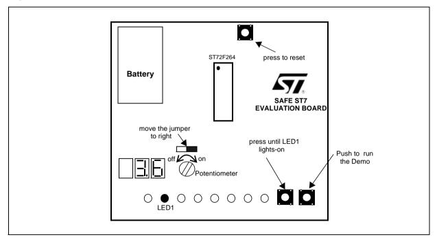
The W3 jumper must be moved to the right to select the variable power supply. If the RV1 trimmer is turned completely clockwise, the board is powered by 5.6 Volts. If the trimmer is turned counter-clockwise the  $V_{DD}$  value will decrease until we reach the LVD threshold ( $V_{IT}$ ), at which point the microcontroller enters reset mode.
