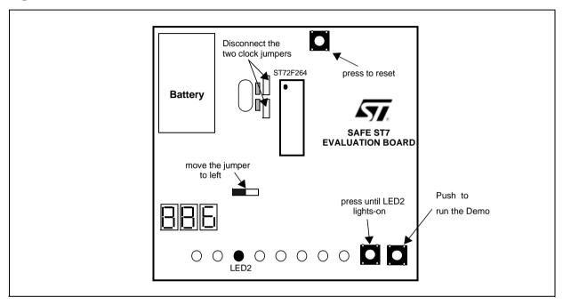
If the clock signal disappears, which you can provoke by disconnecting the two jumpers as shown in Figure 13, the safe oscillator delivers a low frequency clock signal (around 3MHz) for a safe oscillator period which allows the ST7 to save any critical data or perform any kind of emergency operations while the CPU is still running.
