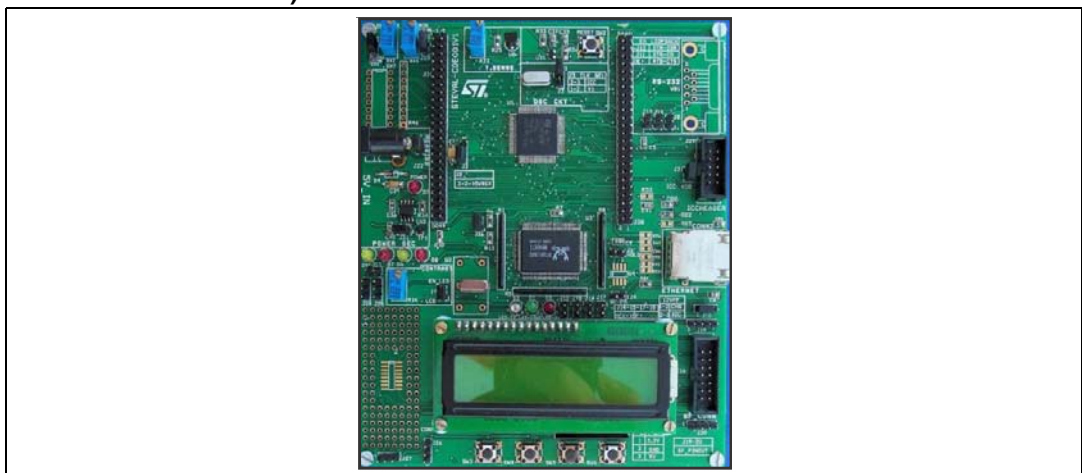
Figure 1. ST72321M9 embedded web server board (order code: STEVAL-CDE001V1)
