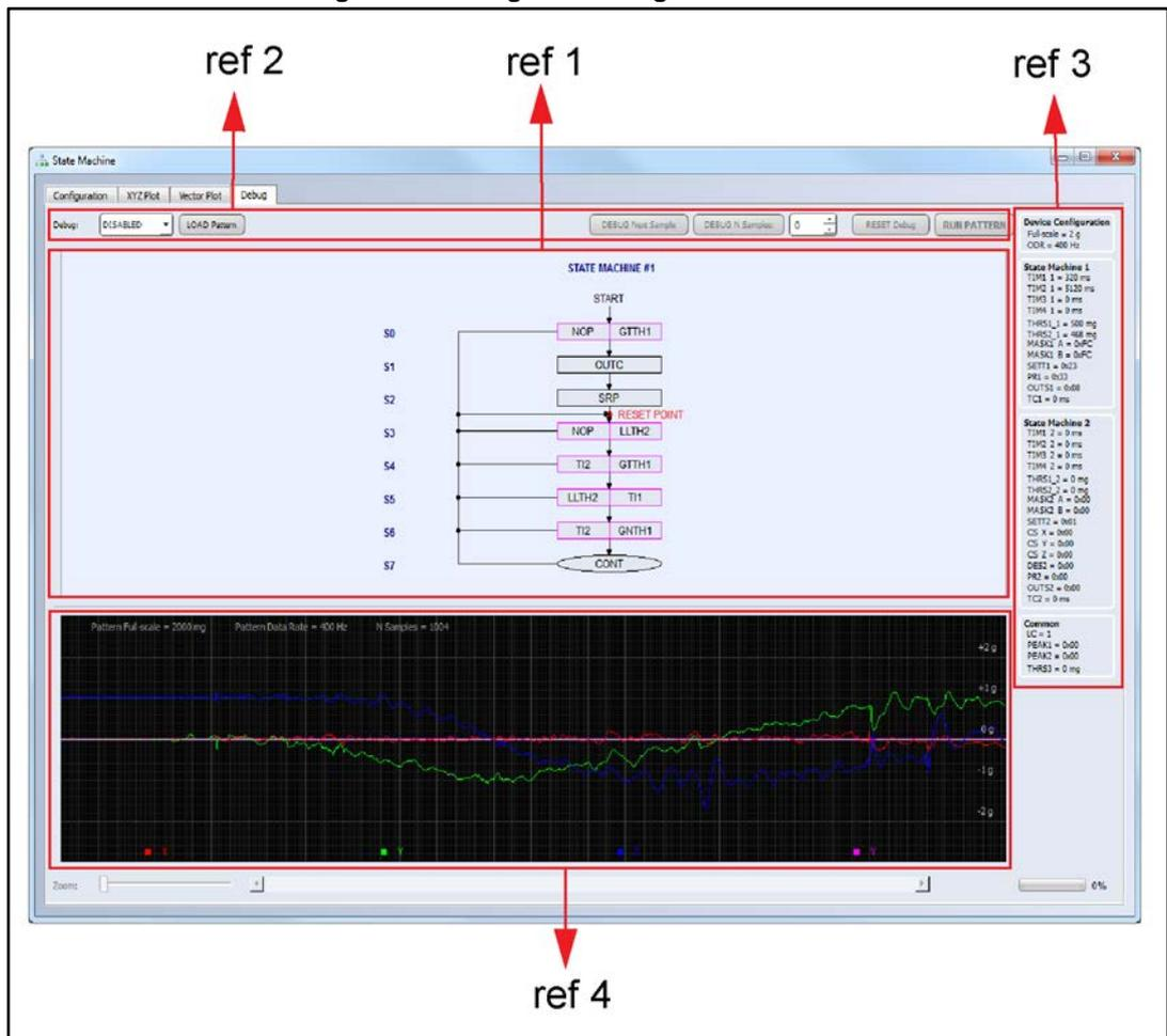
Once the debug mode has been enabled (Figure 17: "Debug tab - Debug mode enabled", ref 1), samples can be loaded by using the controls at the top of the window (Figure 17: "Debug tab - Debug mode enabled", ref 2):
