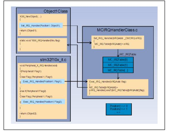
Figure 3: Motor control interrupt handling
