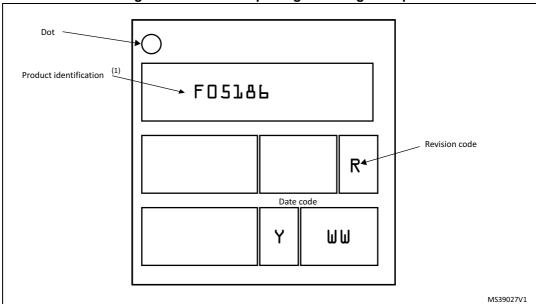
Figure 48. WLCSP36 package marking example
