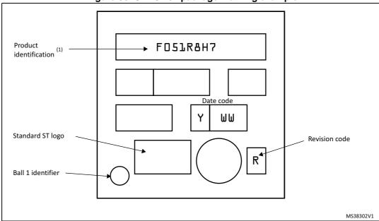
Figure 36. UFBGA64 package marking example
