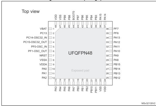
Figure 6. UFQFPN48 package pinout
