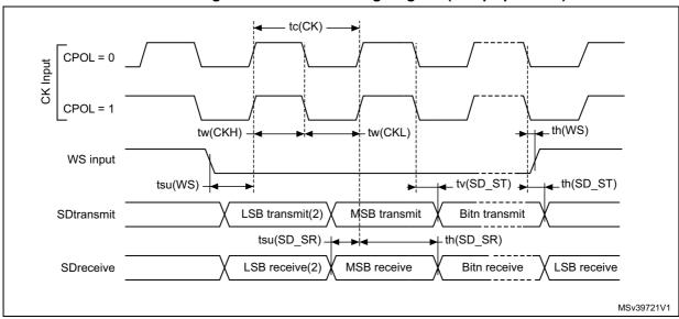
Figure 32. I<sup>2</sup>S slave timing diagram (Philips protocol)
