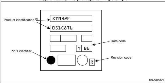
Figure 42. LQFP48 package marking example
