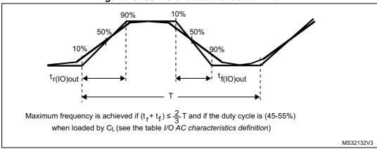
Figure 23. I/O AC characteristics definition
