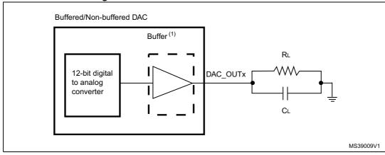
Figure 27. 12-bit buffered / non-buffered DAC
