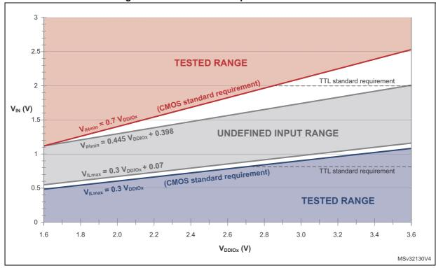
Figure 21. TC and TTa I/O input characteristics
