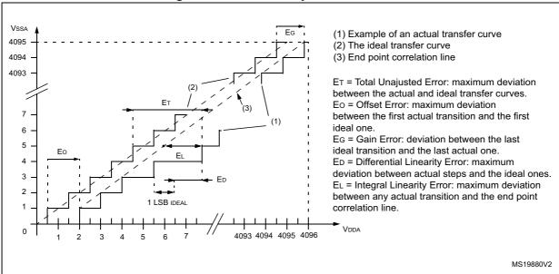
Figure 25. ADC accuracy characteristics
