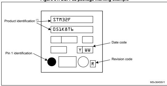
Figure 51. LQFP32 package marking example
