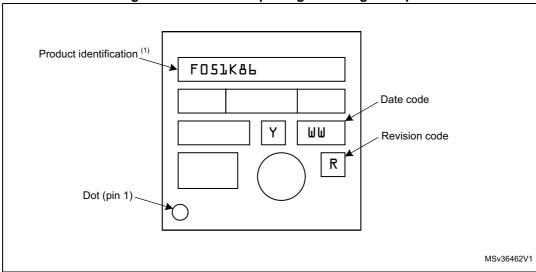
Figure 54. UFQFPN32 package marking example
