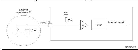
Figure 24. Recommended NRST pin protection
