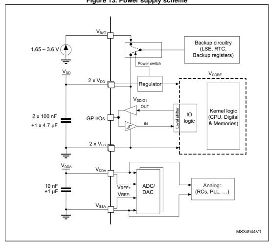
Figure 13. Power supply scheme
