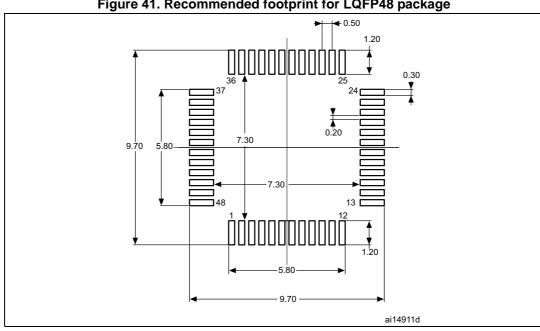
Figure 41. Recommended footprint for LQFP48 package
