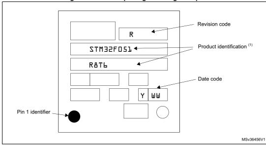
Figure 39. LQFP64 package marking example
