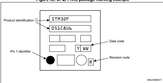
Figure 45. UFQFPN48 package marking example
