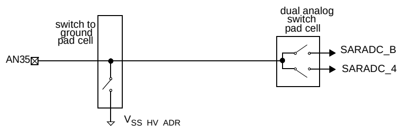
Figure 451. Analog input AN35 — discharge switch to AVSS
