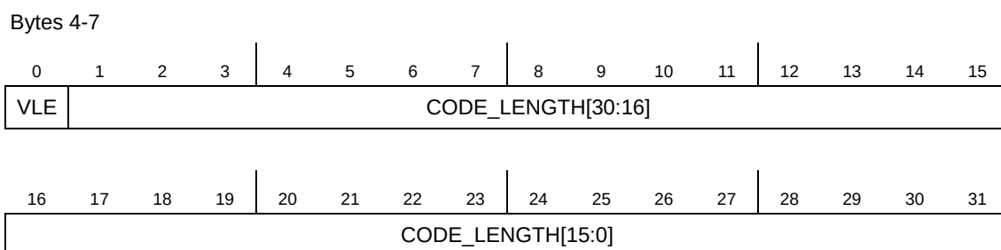
Figure 1424. Download VLE bit and code size
