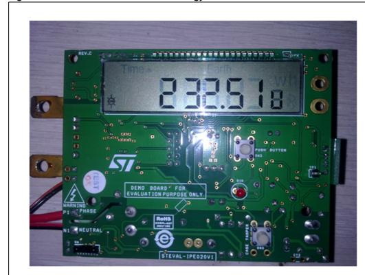
Figure 1. M24LR64 EEPROM based energy meter
