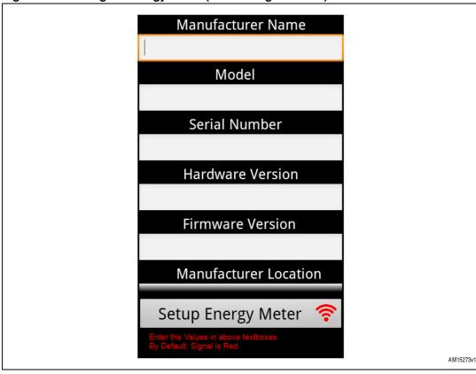
These entries for the configuration of the meter can be done in offline mode and can then be programmed into the dual EEPROM once the phone is brought into range. The signal color changes from red to green.
