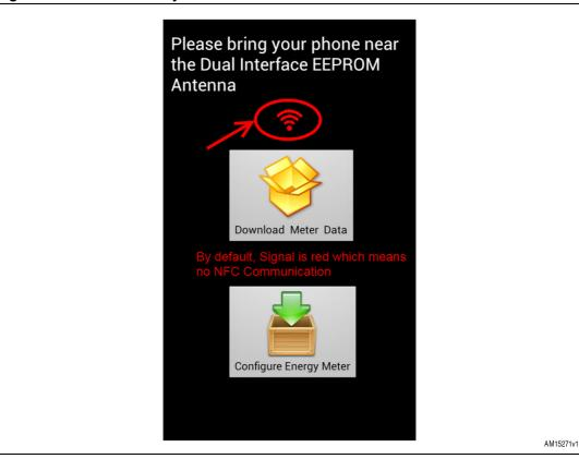
When the user selects the Application button on the main screen of the application, it switches to the screen shown in *Figure 4*. The red signal indicates that no NFC tag was detected by the application. The user needs to bring the phone into the NFC range.
