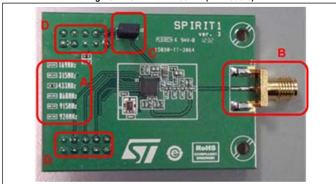
Figure 12. STEVAL-IKR001Vx (RF module)
