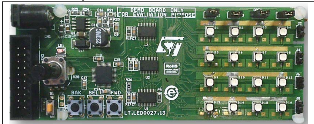
Figure 26. STEVAL-ILL061V1 evaluation board
